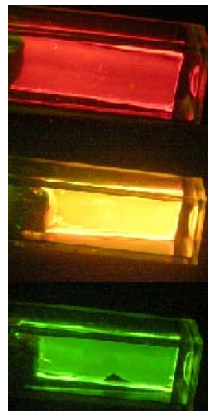
Figure shows thin, spin-coated ethyl cellulose films of our sensor, when irradiated with ultra-violet light (366 nm), under different ambient concentrations of oxygen (from top to bottom: 0, 50-10%, 30-100% O 2 ) [ref 4].
